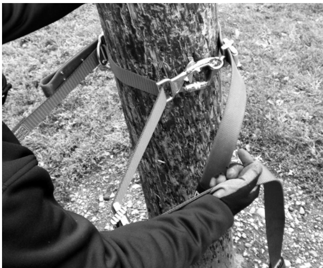
Figure 23 - Adjust Forward into Pole, Web Version
