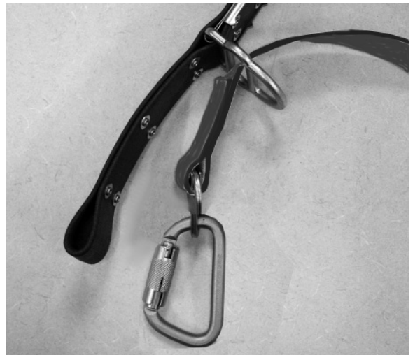
Figure 42 - Support Carabiner Properly Attached to Web Lanyard
