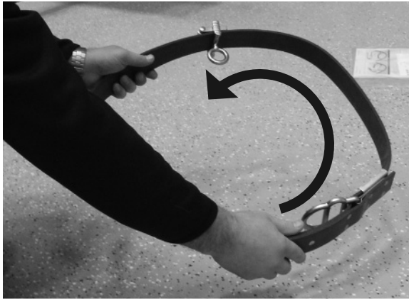
Figure 53 - Rope or Web Lanyard, Flip the strap over so that the Cynch-Lok Roller Adjuster is on the left side
