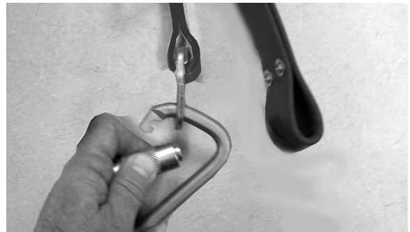
Figure 60 - Connect Body Support Carabiner to Web End
