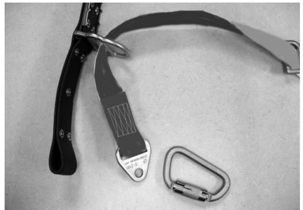
Figure 33 - Disconnect Body Support Carabiner from the Web Lanyard
