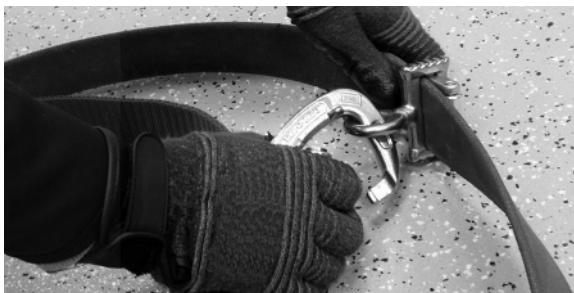
Figure 56 - Web or Rope Model, Attach Captive Eye Carabiner to Cynch-Lok Roller Adjuster
