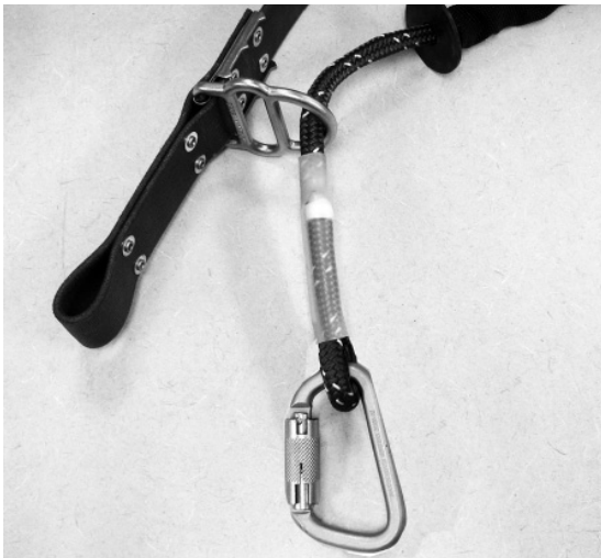
Figure 41 - Support Carabiner Properly Attached to Rope Lanyard
