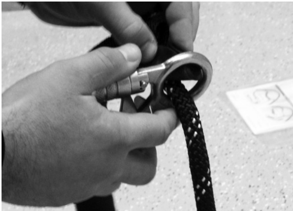
Figure 51 - Remove Captive Eye Carabiner from Rope Lanyard
