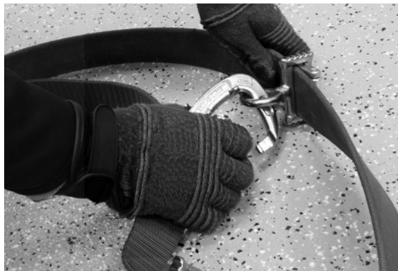
Figure 36 - Rope or Web Lanyard , Disconnect Captive Eye Carabiner from Cynch-Lok Roller Adjuster
